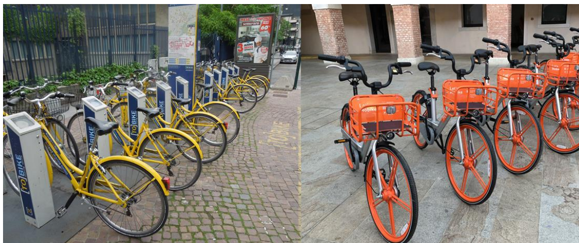
Figura 6. Bike sharing station-based (sx) e free-floating (dx) a Torino - elaborazione da fonti web
